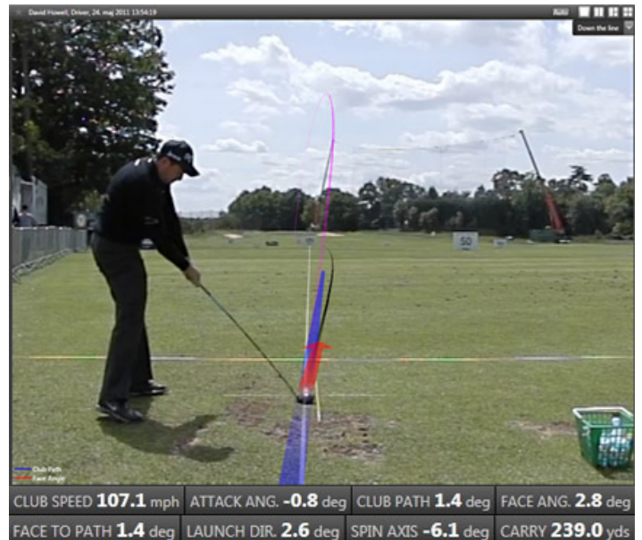
Figure 2. Face-to-Path open with slight toe impact, resulting in a draw
